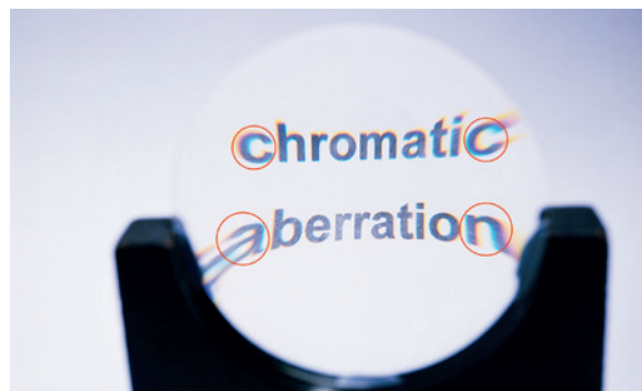
FIGURE 3.2.3 Chromatic aberration causes the coloured fringes that can be seen in the circled regions in this image.
